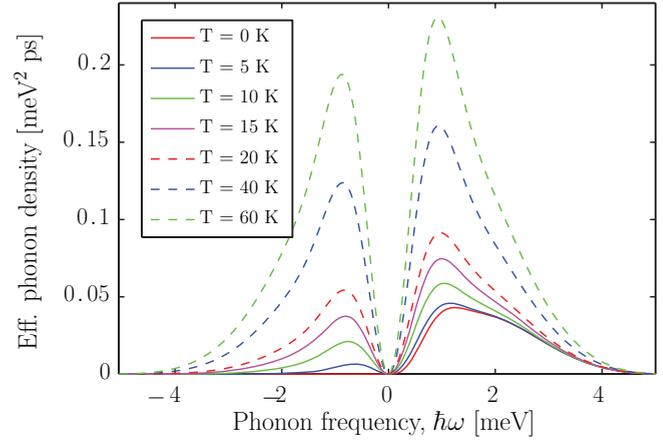
FIG. 6. (Color online) Effective phonon density  $\text{Re}[D^>(\omega)]$  [see Eq. (56)] for a set of temperatures. The weak shoulder visible at low temperatures near  $\hbar\omega \sim 2 \text{ meV}$  arises due to different localization lengths for the electron in the excited and ground states.
