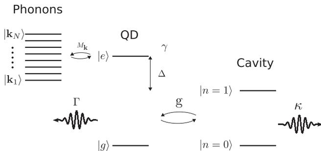
FIG. 1. Schematic of the cavity QED system including the phonon interaction. The QD-cavity coupling strength is  $g$  and the QD-phonon interaction matrix elements are  $M_k$ . The rates  $\Gamma$  and  $\kappa$  yield decay of the QD and cavity, respectively. Pure dephasing of the QD is included through  $\gamma$  and  $\Delta$  is the QD-cavity detuning.
