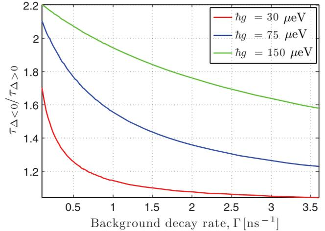
FIG. 9. (Color online) Degree of asymmetry as a function of QD background decay rate. The detuning is fixed at  $\hbar|\Delta| = 1$  meV, while the light-matter coupling strength is varied. Other parameters are  $T = 0$  K,  $\hbar\kappa = 100 \mu\text{eV}$ , and  $\hbar\gamma = 0 \mu\text{eV}$ .
