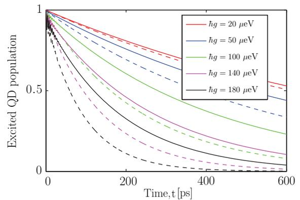
FIG. 7. (Color online) QD decay curves for an initially excited QD. The curves are for different values of the light-matter coupling strength  $g$  with the solid (dashed) lines being for a detuning of  $-1$  ( $+1$ ) meV. Parameters:  $T = 0 \text{ K}$ ,  $\hbar \kappa = 100 \mu\text{eV}$ ,  $\Gamma = 1 \text{ ns}^{-1}$ , and  $\hbar \gamma = 0 \mu\text{eV}$ .
