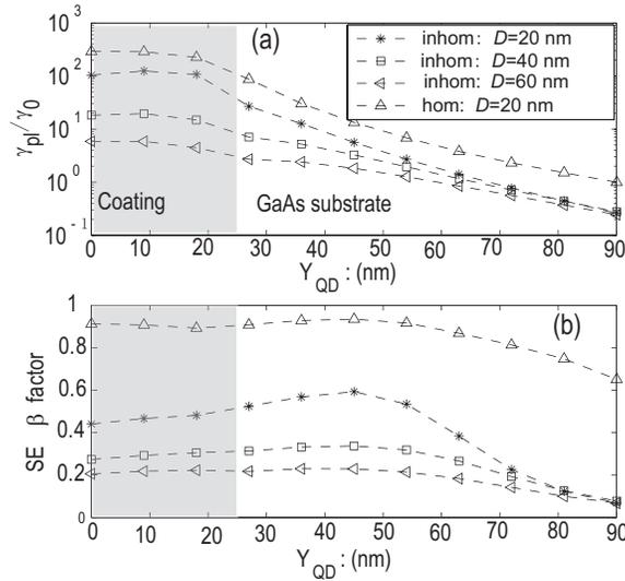
Fig. 5. Position dependence of the plasmonic decay rates and SE  $\beta$ -factors for the metallic slot waveguide with inhomogeneous environment ( $n_c = 1.5$ ,  $n_s = 3.5$ ) and the homogeneous case ( $n_c = n_s = 1.0$ ) with  $X_{QDs} = 0$ ,  $H = 40$  nm,  $W = 100$  nm.
