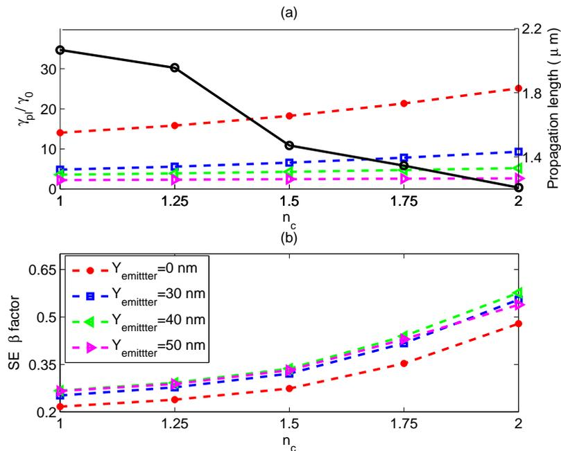
Fig. 6. Role of inhomogeneous environment, quantified by variation of plasmonic decay rate and SE  $\beta$ -factor with  $n_c$  for fixed  $n_s = 3.5$ ,  $X_{\text{QDS}} = 0$ ,  $H = 40$  nm,  $W = 100$  nm,  $D = 40$  nm. The black line shows the propagation length of the gap mode.
