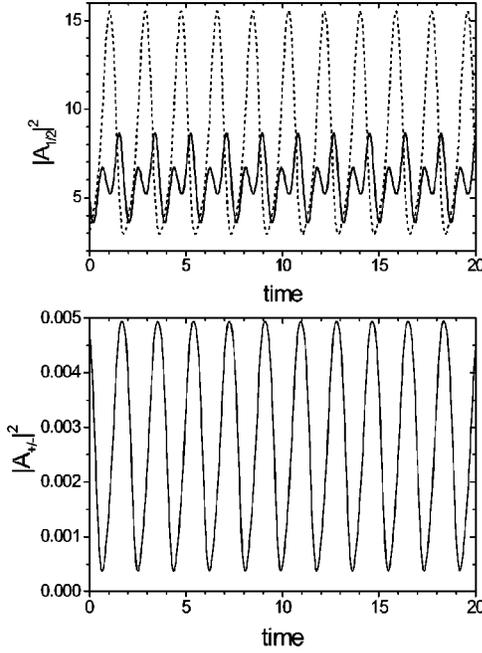
FIG. 2. Self-pulsing solution for all four cavity fields with  $\Delta_1 = -2.5$ ,  $\Delta_2 = 1.2$ , and  $\gamma = 1$ . The pump level is  $E = 11.7$ . The plots display the scaled intensity in the four beams as a function of time. The upper plot shows the fundamental (solid) and second-harmonic (dashed) intensities, while the lower plot shows the parametric intensities.
