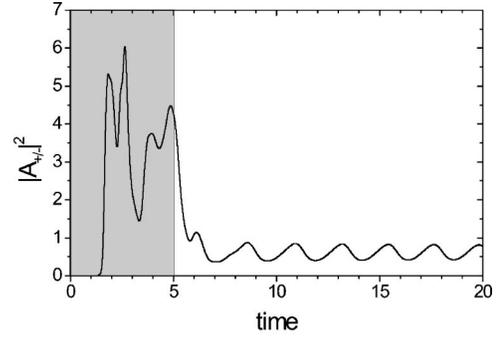
FIG. 9. Self-pulsing cavity solitons for  $E = 62.0$  and the parameters in Fig. 6. The plot shows the average intensity of the parametric fields as a function of time. The gray area indicates the first five time units of the simulation where the address beam is on with a value of  $E = 84.0$ .
