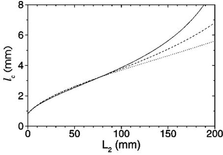
FIG. 13. The spatial scale of the transverse instability as a function of the length of the second harmonic arm  $L_2$ . The lengths of the fundamental arm are  $L_1=10$  mm (solid),  $L_1=20$  mm (dashed), and  $L_1=50$  mm (dotted). The parameters are as in Fig. 10 and with  $\bar{\Delta}_2 = -1.5$ .
